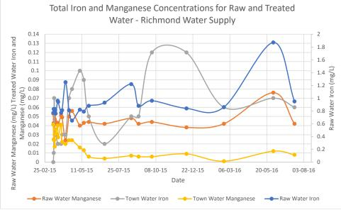
Figure 13.4 Raw and treated water Iron and Manganese for the Richmond Water Supply
