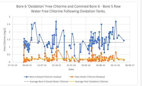
Figure 13.1: Oxidation free chlorine monitoring – Richmond Water Treatment Plant.
